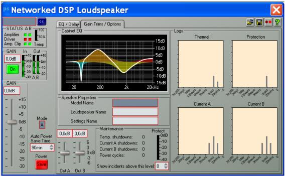
Figure 3: Software of DSP control - Monitoring panel
