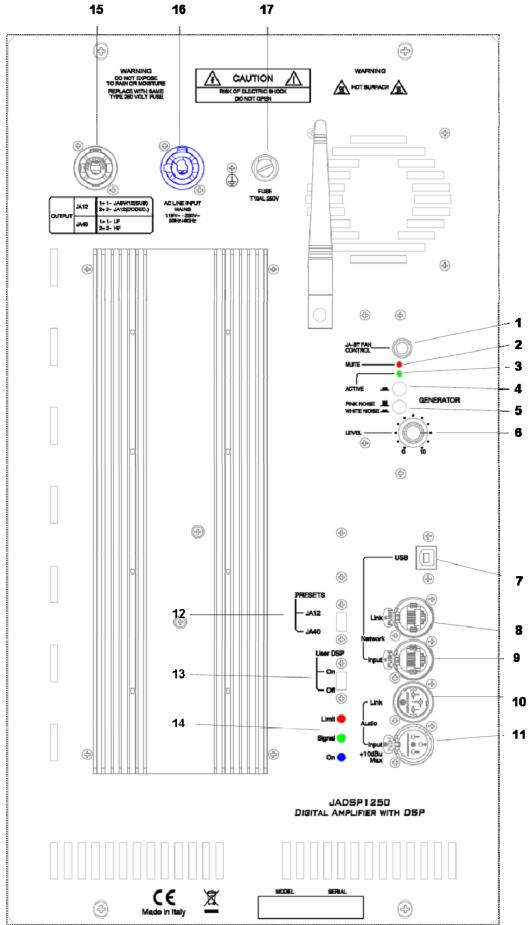
Figure 2: JADSP1250 front panel and numbered scheme
