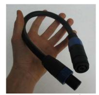
Figure 6: Adapter cable for JA12
