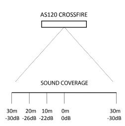
With the revolutionary AS120 Crossfire system, the drop in sound level at 10 metres from the centre of the floor is already -22 dB and at 30 metres can be as much as -30 dB.
