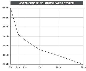
The above diagrams clearly illustrate the significant reduction in sound level that can be achieved outside the floor by using the AS120 Crossfire system instead of a traditional speaker. Measurements by STUDIO ESA (Florence)
