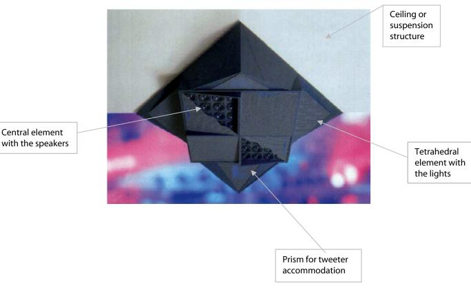
Figure 6. AS120 Crossfire acoustic loudspeaker system
