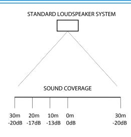
With a standard loudspeaker system, the sound level at 10 metres from the centre of the floor drops by just -13 dB and at 30 metres by -20 dB.
